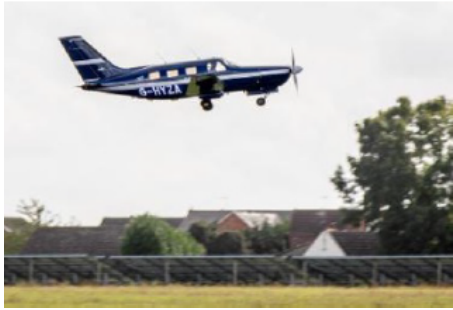
Six-seater Piper Malibu M350 first flight in Sept with ZeroAvia's hydrogen powertrain.
